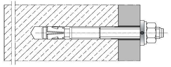
Installation condition with cap nut HM (optional with filling washer)
