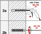
Starting from the bottom or back of the drill hole, blow out the hole with compressed air (min. 6 bar) a minimum of **two** times until return air stream is free of noticeable dust.
