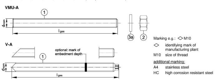
Threaded rod VM-A (material sold by the metre, to be cut at the required length) M8, M10, M12, M16, M20, M24, M27, M30 (zinc plated, A2, A4, HCR)
