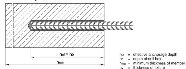
Injection System VMH for concrete
