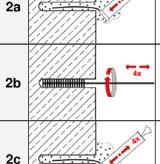
Starting from the bottom or back of the drill hole, blow out the hole with the blow-out pump a minimum of **four** times until return air stream is free of noticeable dust.
