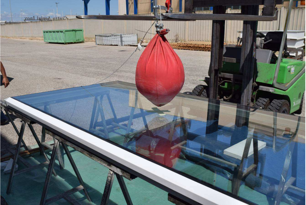
Photo 1. Tested sample in the experimental setup for resistance to large soft body impact
